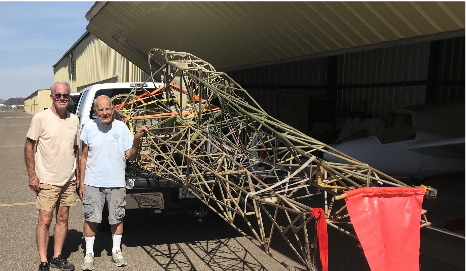
Above is another 'Ridge' refurbishment: making #212, a 1-26B, airworthy again.
