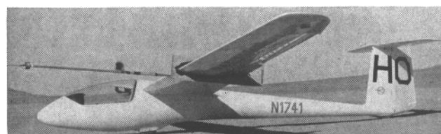
The Phoebus A wearing the swivel airspeed head.
