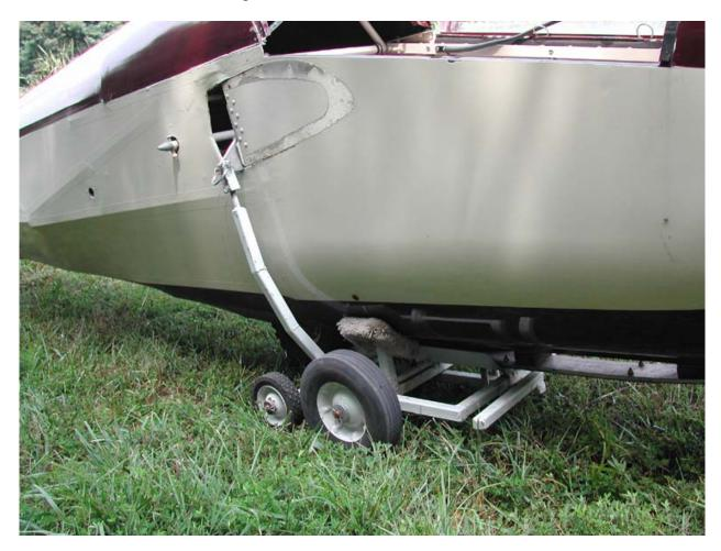
6. A foot operated lever with a roller wheel in contact with the skid lifts the skid up from the dolly channel and permits the fuselage to be up from the dolly. The roller wheel lever applies about a 10 to 1 mechanical advantage, so you will be exerting about 40 pounds of force to lift the fuselage from the dolly. This allows the fuselage to clear the two saddle pads and the channel that supports the skid. The picture shows the lever lifting the fuselage.
