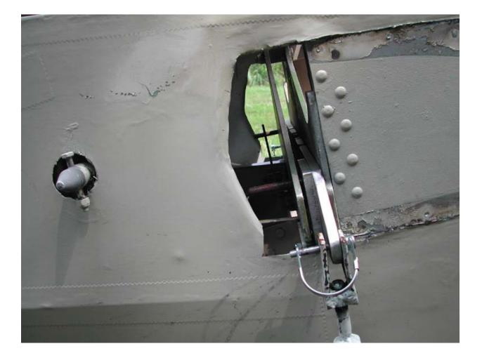
4. Two restraining arms are attached to the carry through bar with quick release pins or tractor pins. The arms swing clear of the lower surface of the wing when the wings are attached. This permits the fuselage to be rolled off of the dolly without making contact with the wings or fuselage.
