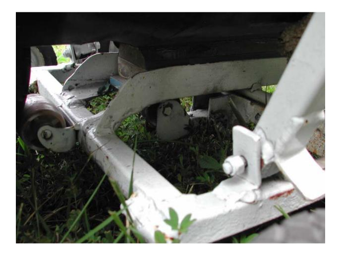
2. The dolly is equipped with two 4x4 inch pads that hold the fuselage upright when the wings are not installed and the restraining arms are not connected. This permits the fuselage to stand alone after both wings have been removed. However, it also means that you will need a wing stand to hold the one installed wing if you want to make this a two man operation. The pads should not be in direct contact with the fuselage. You don't want any friction when you roll the fuselage off of the dolly.
